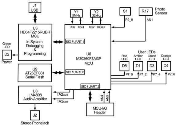
Figure 6-2: HTS Demo Kit Block Diagram
